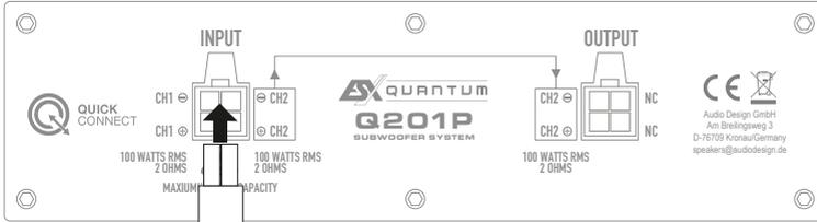
The purple-black and purple cable has no function in this connection example. Both are only needed if another subwoofer system is connected to **OUTPUT** (see below). To be on the safe side, insulate the two loose cable ends.
