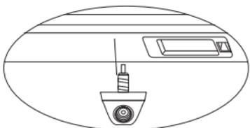
Put the cable and the thread through the hole and fasten the camera with its ring and screw nut.
