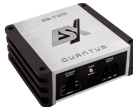
ESX QS-TWO 2-channel Class D Nano Digital Amplifier 2 x 52/95 Watts RMS @ 4/2 Ohms Dimensions: 70 x 35 x 90 mm
