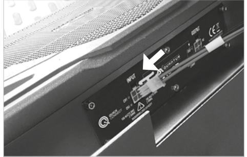
Connect all required connection cables to the subwoofer system as described on pages 8 and 9.
