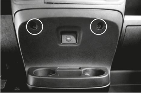
Loosen the two screws (Torx T25) above the cup holder.
