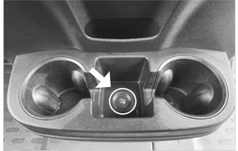
Remove the rubber insert in the center of the cup holder. Then loosen the screw (Torx T25) in the middle.
