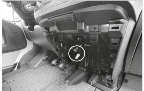
If present, pull out both connector plugs on the console and remove them completely.
