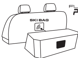
OPTION 1 Bassreflex port rear Sound transmission through the ski bag
